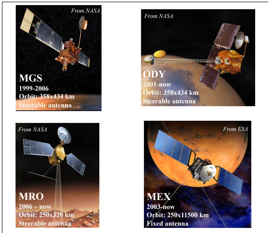
Figure 14: Martian spacecraft used for the determination of the gravity field of Mars and of its moons: Mars Global surveyor (MGS), Mars Odyssey (ODY), Mars Reconnaissance Orbiter (MRO) and Mars Express (MEX).
