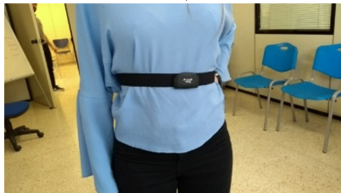
Figure 1. Biosensor placed at the thoracic level to record heart rate variability.
