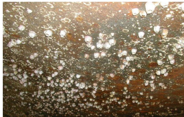
Figure 8. A photo on partial coverage by a colony of barnacles on a biofouled surface ( https://www.marineinsight.com accessed on 25 February 2022).
