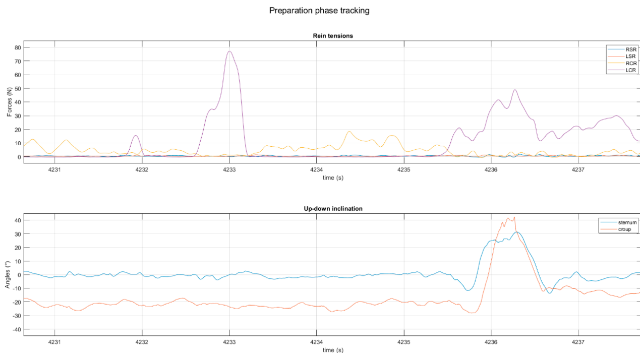
Figure 2. (Top) tensions of left curb rein (LCR), right curb rein (RCR), left snaffle rein (LSR), right snaffle rein (RSR), and (bottom) sternum and croup inclination angles. For the sternum, a positive inclination angle can be equated with a nose-down orientation and a negative inclination angle can be equated with a nose-up orientation of the forehead. For the croup, a negative inclination angle can be equated with a croup-down orientation. The two blue dotted lines mark the preparation phase (from the end of the peak LCR tension to the beginning of the rotation of the forehead) of a croupade.
