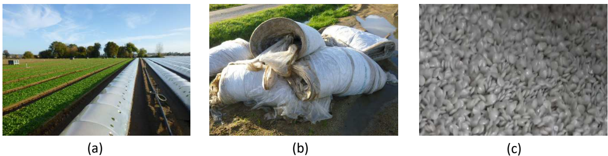
Image 1. (a) Plastic tunnels in use and field after their removal, (b) Films removed, and (c) regenerated pellets (Authors).
