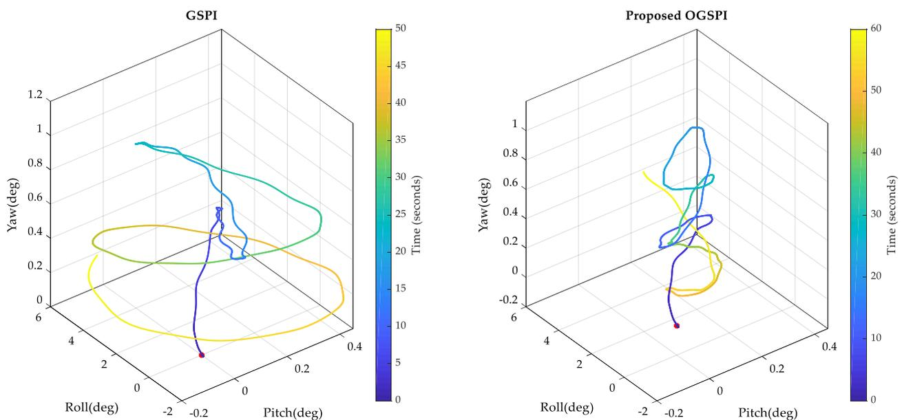
**Figure 9.** The platform inclinations using: (right)—GSPI; (left)—OGSPi.
