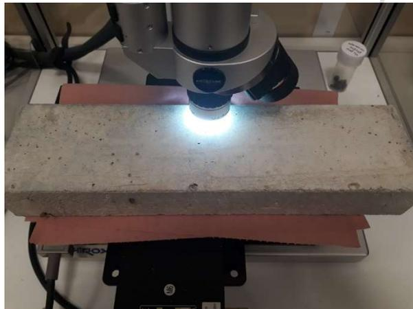
234 **Figure 6.** Photograph of the specimen observation under the optical microscope: a)
