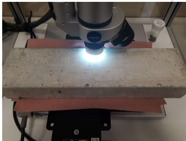
234 Figure 6. Photograph of the specimen observation under the optical microscope: a) 235 global view, b) close-up view of a specimen placed horizontally on top of a paper sheet.
