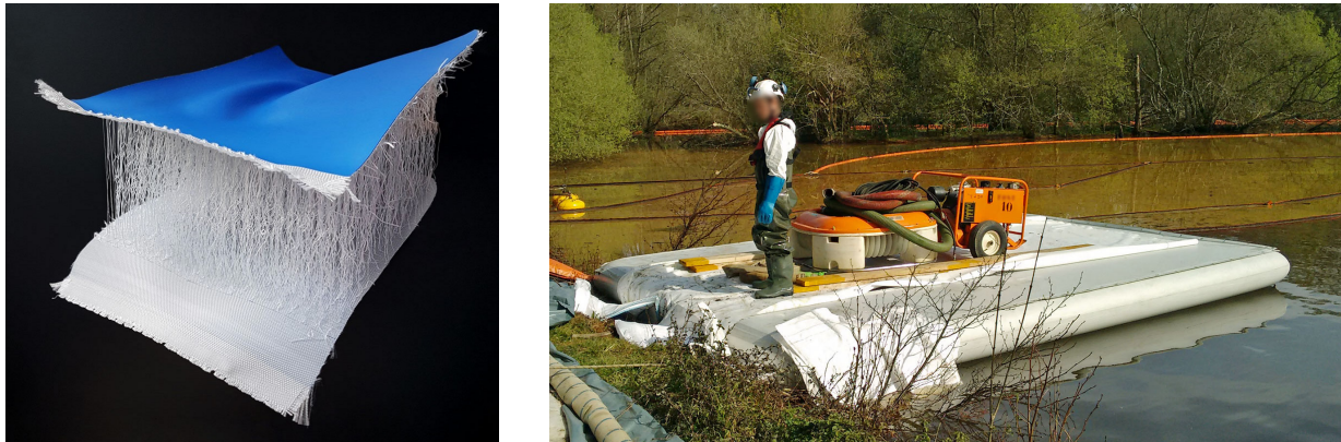
(a) Cut view of drop-stitch fabric exhibiting yarns. (b) Floating decontamination platform. (© Écocréation)
