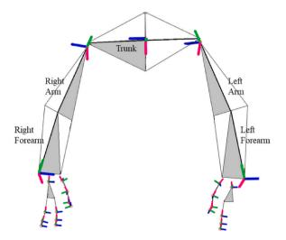
**Fig. 3.** Position and orientation of the segment coordinate system of upper limbs and trunk. Blue axis is for flexion (Z), green is the rotation axis for upper-limb and adduction axis for hand (X), and red is the adduction axis for upper-limb and the axis rotation for hand (Y). In grey the frontal plan from landmarks.
