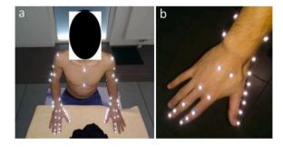
Fig. 2. A. Location of the 52 markers (the marker of the cervical  $n^{\circ}7$  is not visible). b. Location of the 24 markers of the right hand (dominant). The third finger of the non-dominant hand (left) is not equipped.
