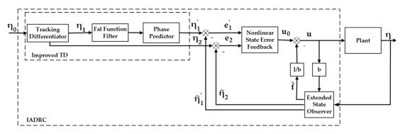
Figure 10. The principle of IADRC.
