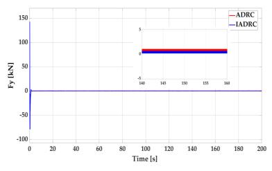
Figure 24. The Force in the sway direction under ideal sea condition.
