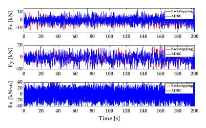
Figure 19. The forces and moment under environmental disturbances.
