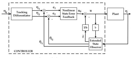
Figure 3. The structure of ADRC [42].
