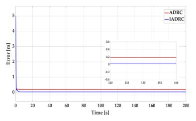
Figure 21. Tracking error under ideal sea condition.
