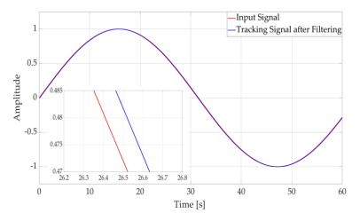
Figure 7. The tracking signal after fal function filter.
