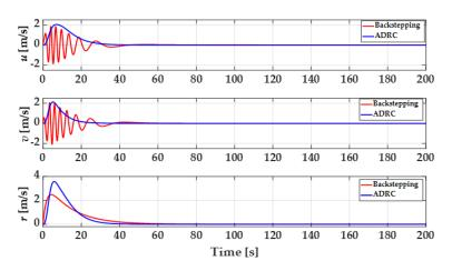
Figure 14. The speed of the ship under ideal sea condition.
