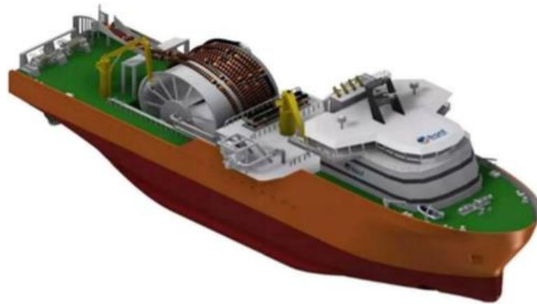
**Figure 1.** A cable laying vessel with DP system [3].
