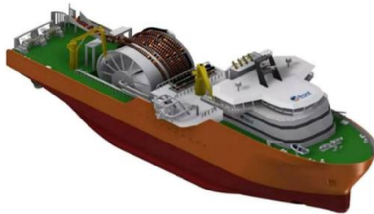
Figure 1. A cable laying vessel with DP system [3].
