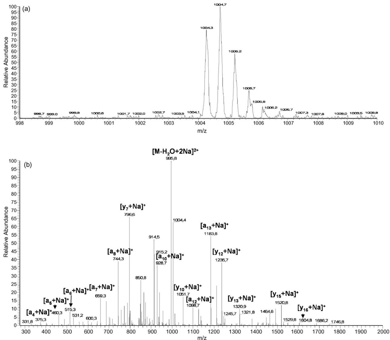
Fig. 2. Mass spectra of alamethicin F50/5: (a) Zoomscan mode; (b) MS<sup>2</sup> spectrum of ion at  $m/z$  1004.3  $[M+2Na]^{2+}$ . The main fragments corresponding to  $a_n$  and  $y_n$  ion series are shown.
