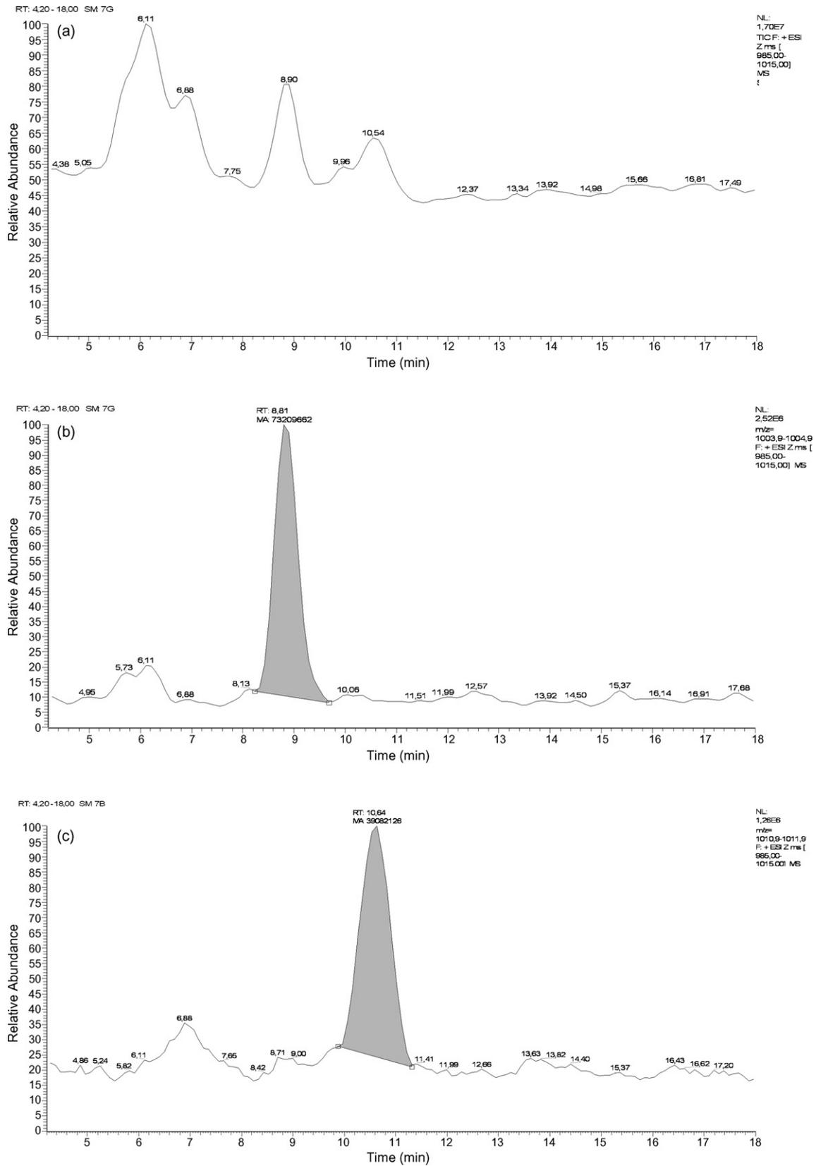
Fig. 3. LC/ESI-IT-MS analysis of surface sediment samples collected from Fiers d’Ars — chromatograms of fraction D spiked with alamethicin F50 reference solution (25 µg/L): (a) total ion current; (b) detection on the range [1003.9–1004.9]: peak of alamethicin F50/5; (c) detection on the range [1010.9–1011.9]: peak of alamethicin F50/7.
