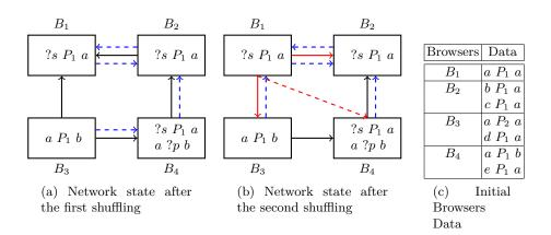
Fig. 2: Partial Snob network centred on  $B_1$ . Solid lines represent clients in RPS view. Dashed lines represent clients in SON view. Each client has a profile with a list of triple patterns representing its running queries.
